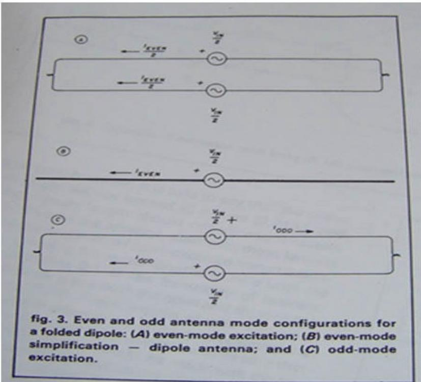
fig. 3. Even and odd antenna mode configurations for a folded dipole: (A) even-mode excitation; (B) even-mode simplification — dipole antenna; and (C) odd-mode excitation.
