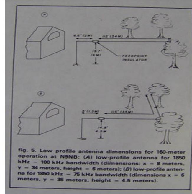
fig. 5. Low profile antenna dimensions for 160-meter operation at N9NB: (A) low-profile antenna for 1850 kHz - 100 kHz bandwidth (dimensions:  $x = 8$  meters,  $y = 34$  meters, height = 6 meters); (B) low-profile antenna for 1850 kHz - 75 kHz bandwidth (dimensions  $x = 6$  meters,  $y = 35$  meters, height = 4.5 meters).
